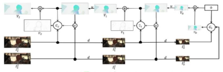
Figure 1. Inference in a 3-Level Pyramid Network [15]: The network  $G_0$  computes the residual flow  $v_0$  at the highest level of the pyramid (smallest image) using the low resolution images  $[I_0^1, I_0^2]$ . At each pyramid level, the network  $G_k$  computes a residual flow  $v_k$  which propagates to each of the next lower levels of the pyramid in turn, to finally obtain the flow  $V_2$  at the highest resolution.
